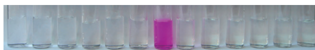
Fig. 3 Color changes observed for 1 (10 \mu M ) in 99 : 1 H_2O-CH_3CN solutions at pH 4.0 (in a 10 mM NaOAc-HOAc buffer) upon addition of 5 \mu M metal ions. From left to right: blank, Ba^{2+} , Cr^{3+} , Cu^{2+} , Co^{2+} , Cd^{2+} , Hg^{2+} , Ag^+ , Fe^{3+} , Zn^{2+} , Pb^{2+} , Ni^{2+} , Mn^{2+} .
